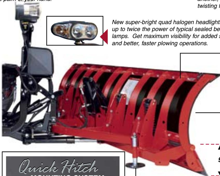
30-inch tall, high curve, high-density polyethylene moldboards are dent-resistant and corrosion-free. Snow flows easily for more efficient plowing.
